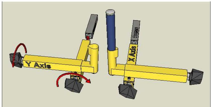
Here are the two different ways the adjuster can be set up. The adjuster on the left is set up for typical counter clockwise lathe rotation. The rig on the right is set up for reverse lathe rotation
