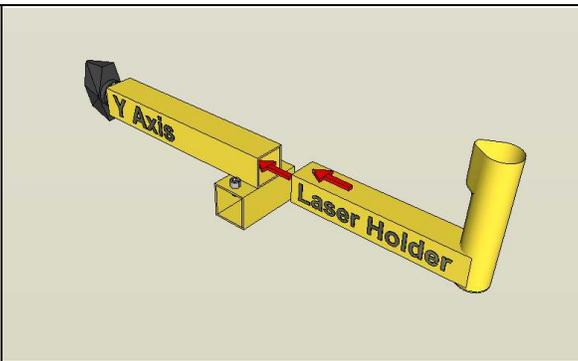
Slide the **Laser Holder** into the **Y-Axis** until it hits the end of the lead screw
