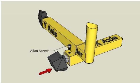
Continue slipping the two parts together until the set screw holes line up. Install and snug up the **Allan Screw**.
