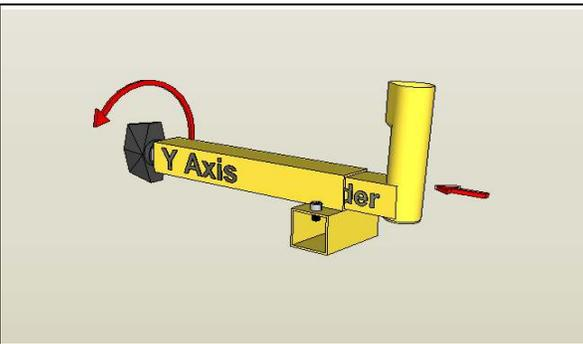
Turn the lead screw counter clockwise while pushing in on the **Laser Holder** until the lead screw engages the captured nut of the **Holder**. Continue turning the knob until the **Holder** is retracted most of the way into the **Y-Axis**
