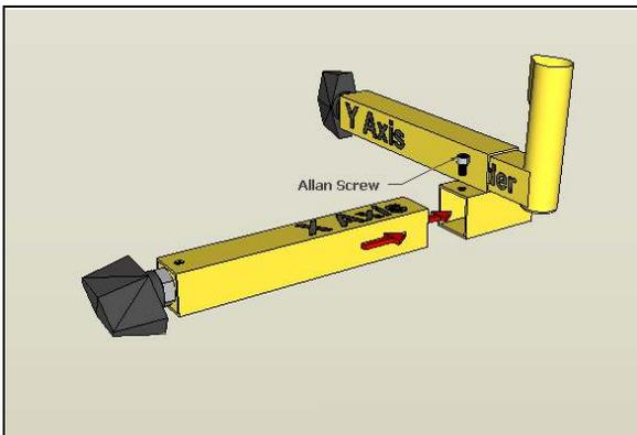
Line up and then slide the **X-Axis** into the sleeve of the **Y-Axis**.
