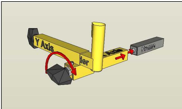
Install the adjuster by sliding the **X-Axis** onto the nose of the **Steel Frame** until it hits the captured nut. Turn the **X-Axis** knob clockwise until the adjuster advances as far as it will go onto the frame.
