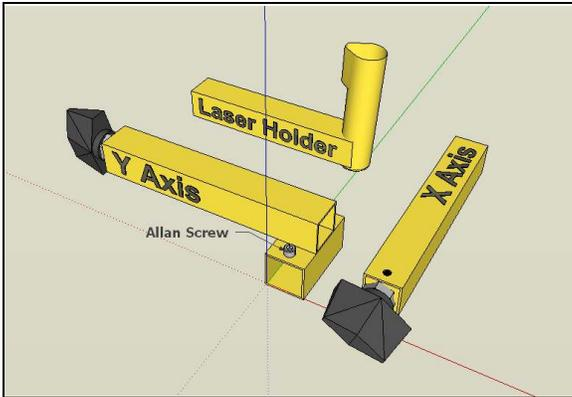
**Please Note:** The system may be assembled so the **Laser** is oriented either on the right side of the tooling or on the left side. This will be dependent on whether you choose to cut with typical counter clock wise (forward) spindle rotation or clockwise (reverse) rotation
